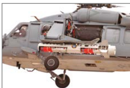
CSTRS winch and tow sheave configuration
