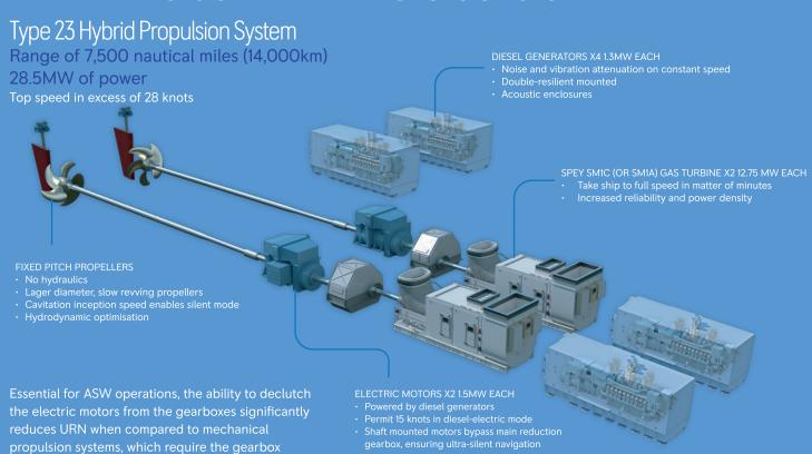
By acoustically enclosing the diesel generators and enabling their physical location above the waterline, the hybrid system further enhances stealth capability to produce ultra-quiet propulsion states.
