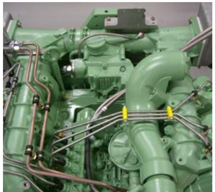
Engine modification for a naval application featuring dual sheathed fuel lines
